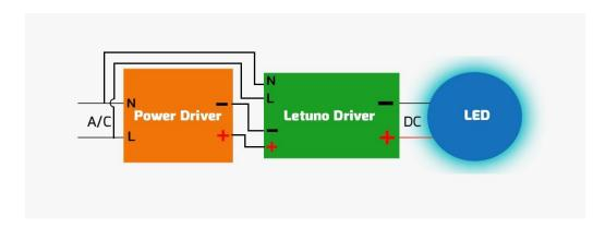
Since the design can power up two lamps in the same circuit, as shown in the below figure the input and the output blocks are specified with the polarity of each side
